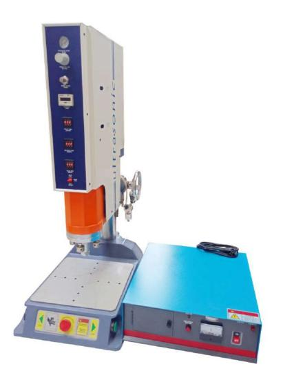
Standard series SE traditional frequency tracking system. The ultrasonic frequency 15 kHz, output power of 3200Watt. Desktop machine with oscillation box (optional purchase station work tables). The ultrasonic welding mold design and production according to the work piece. Equipment for the welding of thermoplastic plastic.
