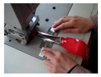
Roller and horn made of special alloy steel, roller's pattern can design by client's requirement, the horn stand wear and tear long using life, easy to replace roller and horn, core shift design, flexible adjusting, easy to adjust the horizontal.
