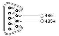
Note: This device uses RS485 communication, baud rate 57600, data format 8/N/1, double-word high and low byte
