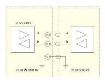
Attention: RS485 communication interface, strong interference occasions using isolation interface, shielding twisted pair.
