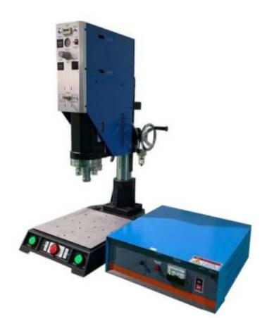
SE standard series Free tone frequency automatic frequency control system.
